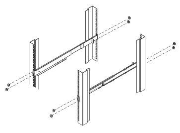
3. Slide the KL1116 onto the support flanges. Use the screws supplied with this package to loosely attach the front of the KL1116 to the front of the rack (only tighten the screws part way).
